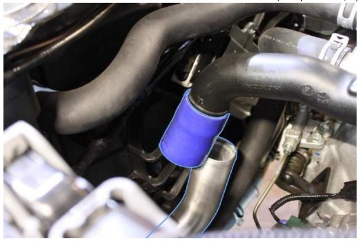
2.10 Align and the piping and tighten all hose clamps and re-install the two mounting bolts, in step 2.8, back onto the upper "cold pipe"
