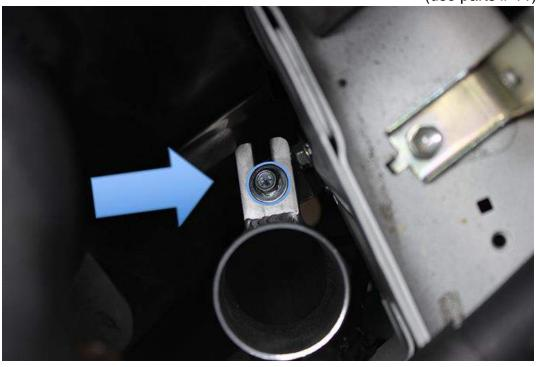
2.6 Next install the upper "hot pipe" I-1 in between the factory plastic turbo outlet and the lower pipe you just installed.
