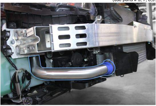
2.5 Attach the provided M6 bolt and washer to secure the lower "hot pipe" I-2 as shown.
