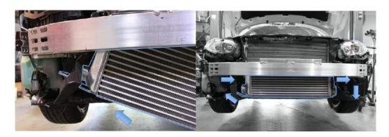
2.3 From underneath, insert the provided M10x40mm bolt up through the lower under frame through the factory intercooler rubber bushing and new Intercooler bracket. \*(Some early kits will have a pre-welded stud that fits into the factory rubber bushing from above, instead of the provided #10. bolt.)
