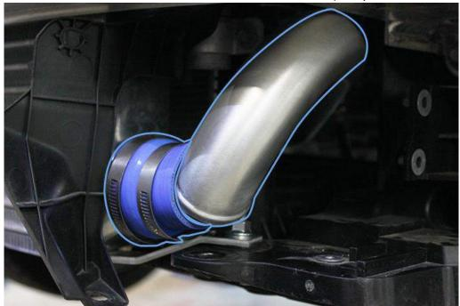
2.8 Temporarily remove the two mounting bolts on the upper "cold pipe", to allow for installation of the new lower "cold pipe" below.
