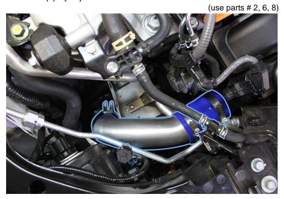
2.7 Install the 50-60 reducer hose onto the Intercooler end-tank and slide the "cold pipe" I-3 into position as shown.
